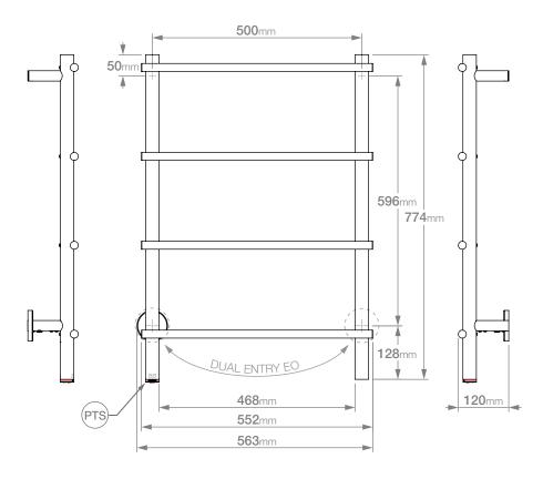
Dimensions given are in **mm**. Bathroom Butler® reserves the right to alter and/or remove designs from time to time without prior notice. This drawing is to be used for reference purposes only. E &O.E.
