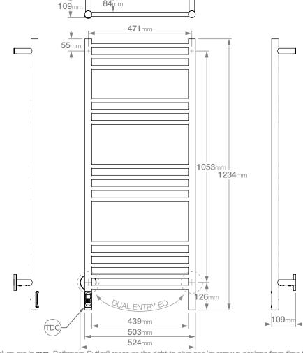
Dimensions given are in **mm**. Bathroom Butler® reserves the right to alter and/or remove designs from time to time without prior notice. This drawing is to be used for reference purposes only. E &O.E.
