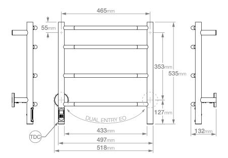
Dimensions given are in mm. Bathroom Butler® reserves the right to alter and/or remove designs from time to time without prior notice. This drawing is to be used for reference purposes only. E &O.E.
