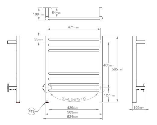
Dimensions given are in **mm**. Bathroom Butler<sup>®</sup> reserves the right to alter and/or remove designs from time to time without prior notice. This drawing is to be used for reference purposes only. E &O.E.
