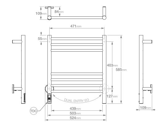
Dimensions given are in **mm**. Bathroom Butler® reserves the right to alter and/or remove designs from time to time without prior notice. This drawing is to be used for reference purposes only. E &O.E.
