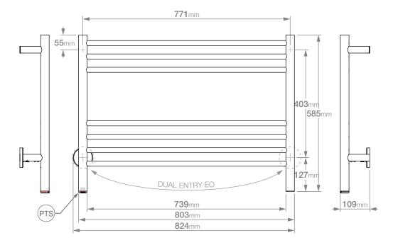
Dimensions given are in mm. Bathroom Butler® reserves the right to alter and/or remove designs from time to time without prior notice. This drawing is to be used for reference purposes only. E &O.E.
