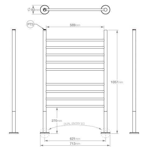
Dimensions given are in **mm**. Bathroom Butler<sup>®</sup> reserves the right to alter and/or remove designs from time to time without prior notice. This drawing is to be used for reference purposes only. E &O.E.
